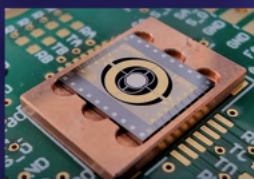
► 2D piezo MEMS \mu -mirror for projection systems
